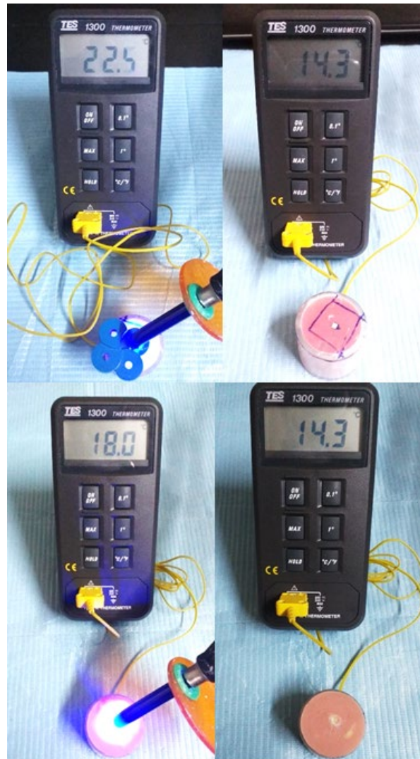
Figure 5: Measurement of temperature rise during stage 1 (upper) and stage 2 (lower) of curing
