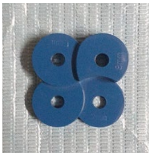
Figure 4: The dimension adjuster used to maintain the distance between the light guide tip and dentin disc
