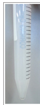
Figure 3: Image of stable translucent 0.5% aqueous dispersion of CNP in test-tube prepared by hydrolysis of cellulose with 40 wt. % SA at 80°C followed by sonication.
