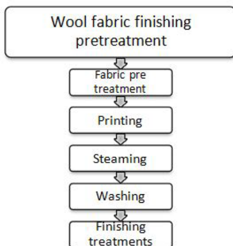
Figure 4: The flow chart of the digital textile printing process for woolen fabrics
