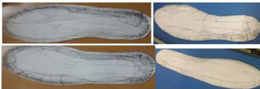
Figure 2: Comparison of (A) Carbon Copy Test Result of Eva and (B) Memory Foam Shoe Insert
