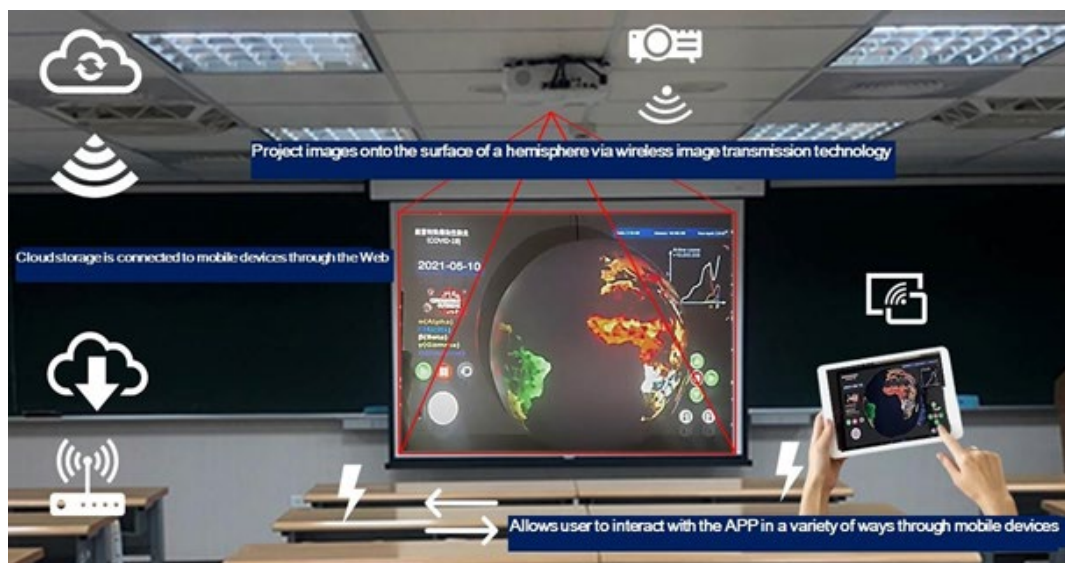
Figure 3: Schematic diagram of the overall architecture of the 3D digital global health information teaching system developed in this work.
