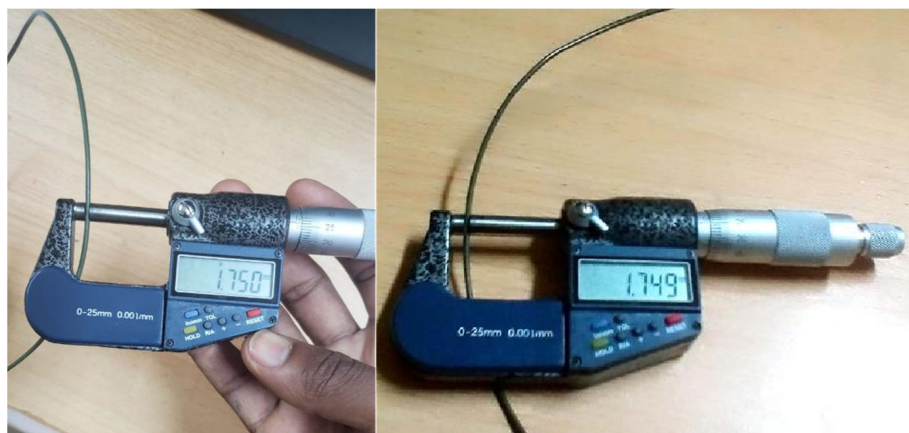
Figure 18: Measuring of the produced recycled HDPE filament diameter at different points
