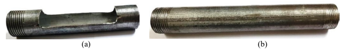
Figure 6: Manufactured barrel: (a) feeding section for hopper installation and (b) heating section
