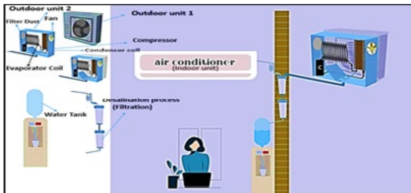
Figure 8: Proposed system design
