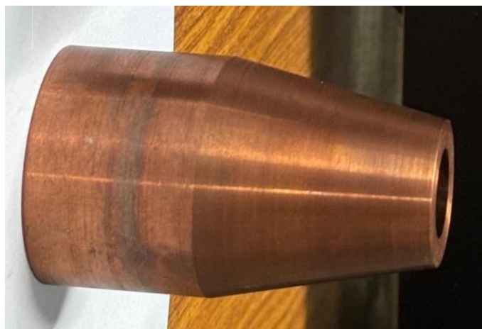
Figure 8: Fabricated Collector by OFHC Copper
