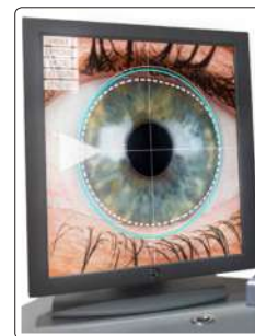
Figure 37: Large color screen to check iris treatment and manage any sudden movement by eye tracking
