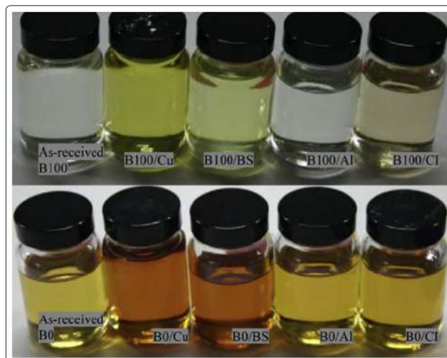
Figure 25: Change in color and compositions of biodiesel and diesel when they exposed to AL, Cu BS and CI [18].
