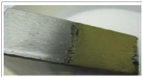
Figure 33: 1018 metal coupon corrosion induced by Moniliella wahieum Y12 in biodiesel as the carbon source. Chemical oxidation of the control coupon after 60 days incubation [22].
