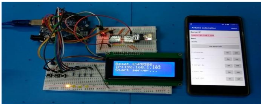
Figure 8: ESP8266 Wi-Fi Module Connection to Microcontroller with Mobile App
