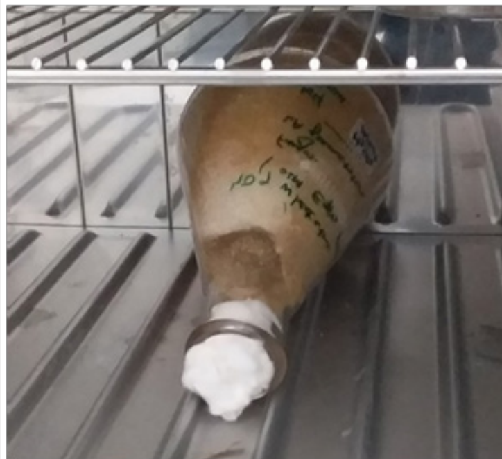
Figure 2. 2: Pretreatment Of Heat Straw By Coriolus Versicolor
