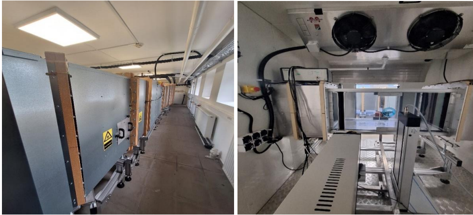
Figure 2: The closed-loop horizontal wind tunnel and its test section.
