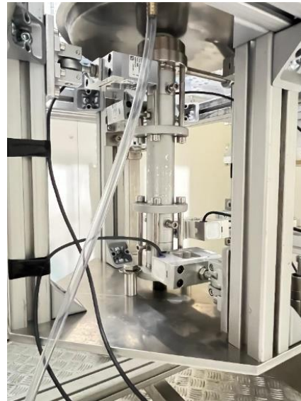
Figure 3: Strain gauges set up used to measure forces acting on the airfoil section.
