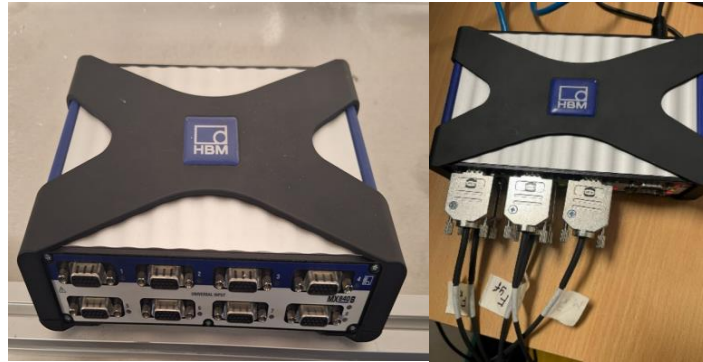
Figure 4: QuantumX MX840B data acquisition system and its connection to the Load cells.
