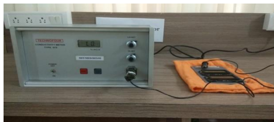
Figure 4: Setup for electrical conductivity measurement
