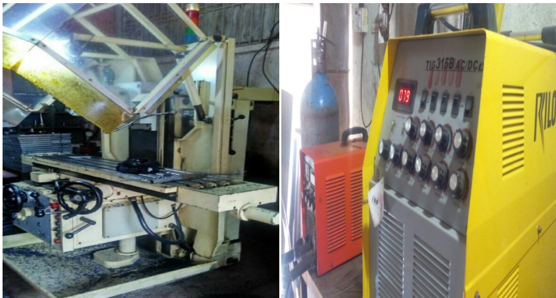
Figure 2: (a) Milling machine used for FSW (b) Machine used for TIG
