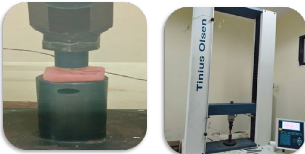
Figure 2: Testing Machine to Assess Push-Out Bond Strength.
