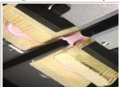
Figure 2: Device under tension. Notice deformation in the walls
