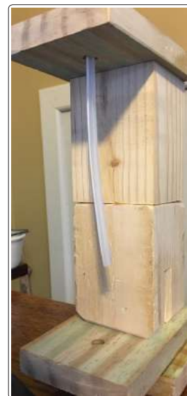
Figure 10: Initial Setup of Elongation Test
