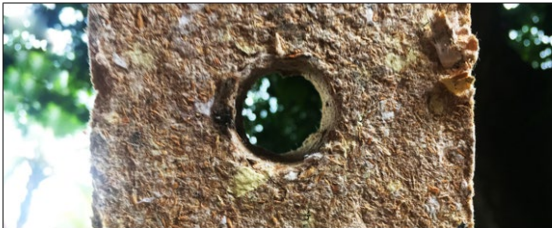
Figure 2. A briquette made of paper, cardboard and sawdust, (El Fuego del Sol, n.d.)
