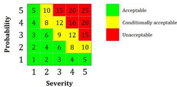
Figure 1: the acceptance criteria for the accumulated risk factor priority number. Three colors of green, yellow and red are symbols for the acceptance, conditionally acceptance and unacceptance of any specific risk for the product
