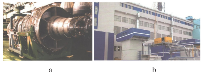
Figure 4: NK-37 gas turbine engine with a capacity of 25 MW, efficiency 36% (a) and gas turbine power station GTE-25 / NK based on the gas turbine NK-37 (b)
