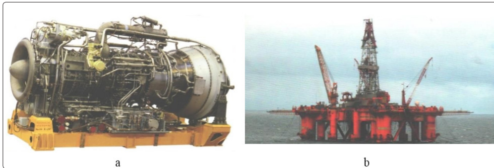
Figure 5: Marine gas turbine engine M75RU, with a capacity of 5.7-10.3 MW, efficiency 33-35% (a) and its application on the drilling platform (b)
