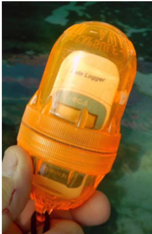
Figure 4: A data logger (Elitech RC-5) is installed at the bottom of the tank, and data is acquired every 30 minutes from 20:00 to 19:30 the next day.
