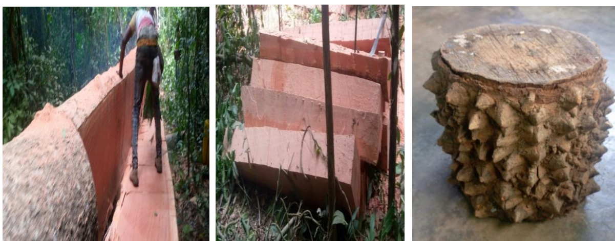
Figure 3: E. cylindricum Stem Cross-Cut into Logs (A), Logs sawn into cants for Easy Transportation (B)
