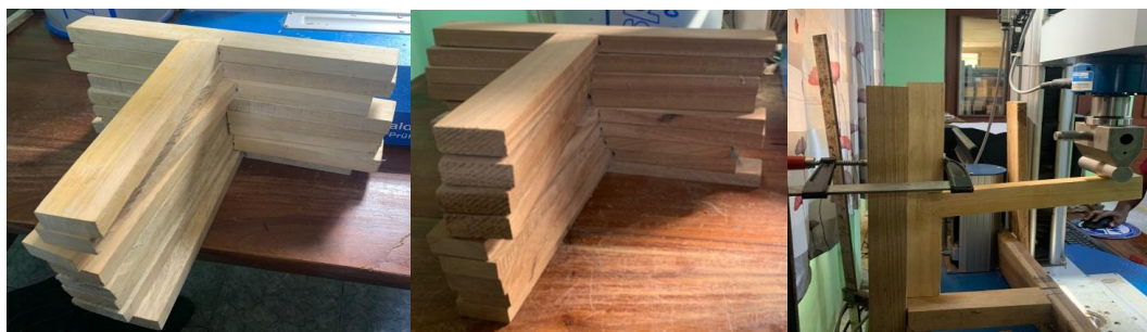
Figure 5: Joints Prepared from Z. Gilletii (1), E. Cylandricum (2) and Sample Under Load on UTM
