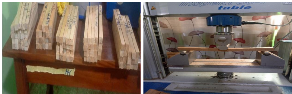
Figure 4: Sample Placed Under Load
