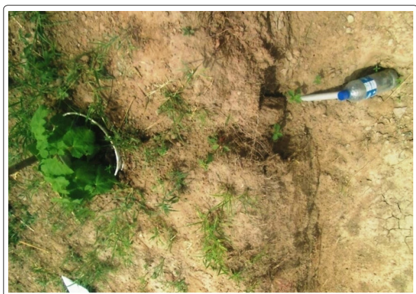
Plate 2: A Unit of the Minilysimeters Showing the Crop Area and the Drainage Collection Point
