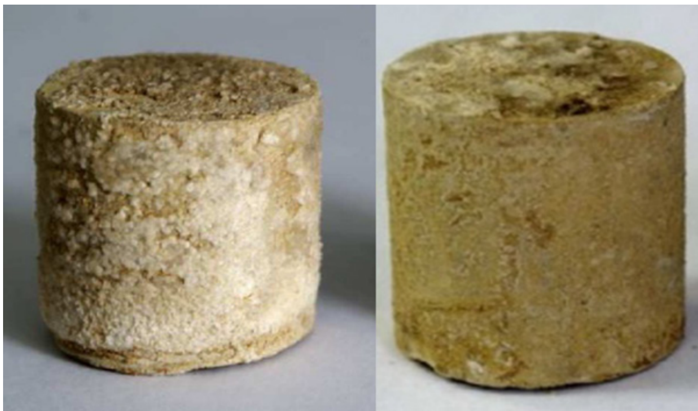
Picture 1: Samples of cement stone based on PCT-1-50 and high alumina cement
