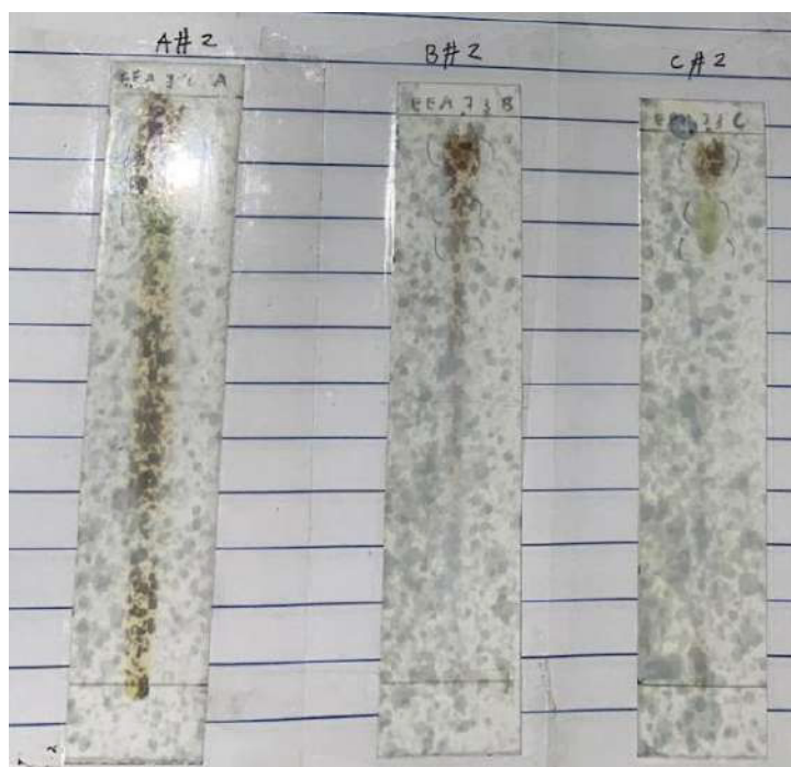
Figure 10. Phytochemical screening results of D. dao , T. catappa , and Z. talanai after spraying Potassium ferricyanide-ferric chloride.
