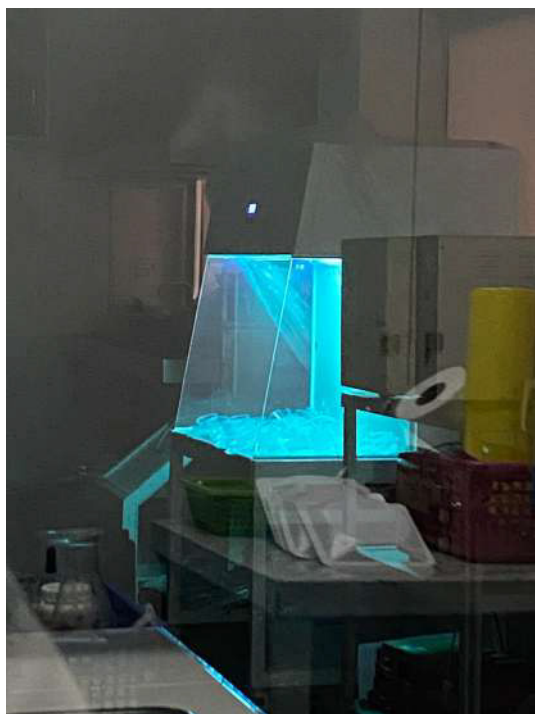
Figure 42. UV sterilization of laminar flow hood
