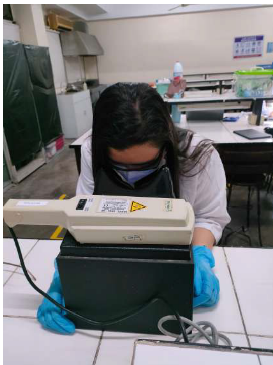
Figure 38. Viewing TLC plates under UV light.
