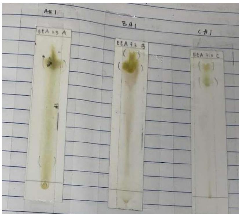
Figure 6. Phytochemical screening results of D. dao , T. catappa , and Z. talanai after spraying Antimony (III) chloride.
