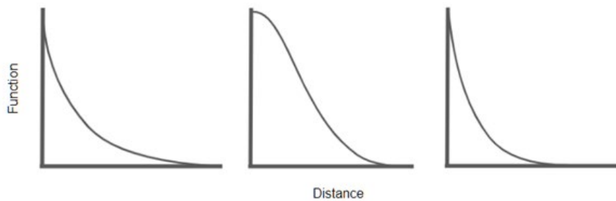
Figure 1: Inverse-power function on the left, Gaussian function in the middle and negative exponential function on the right.
