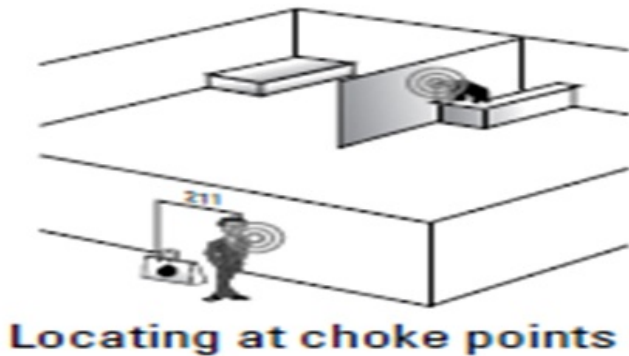
Figure 1: Scenario of using RFID to locate a wandering elderly person at chokepoint.
