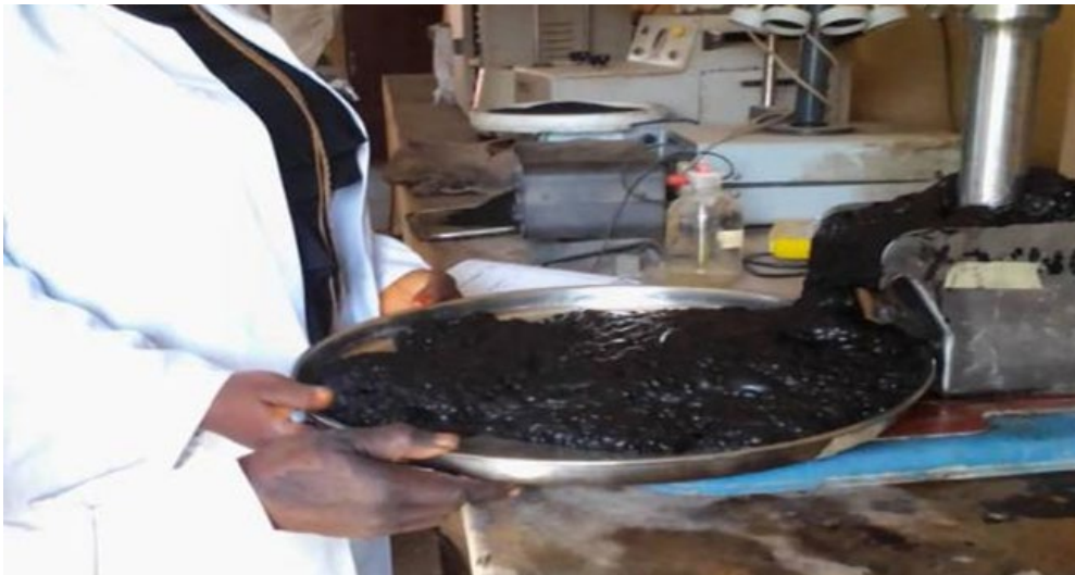
Figure 4: Collection of Resins using froth flotation
