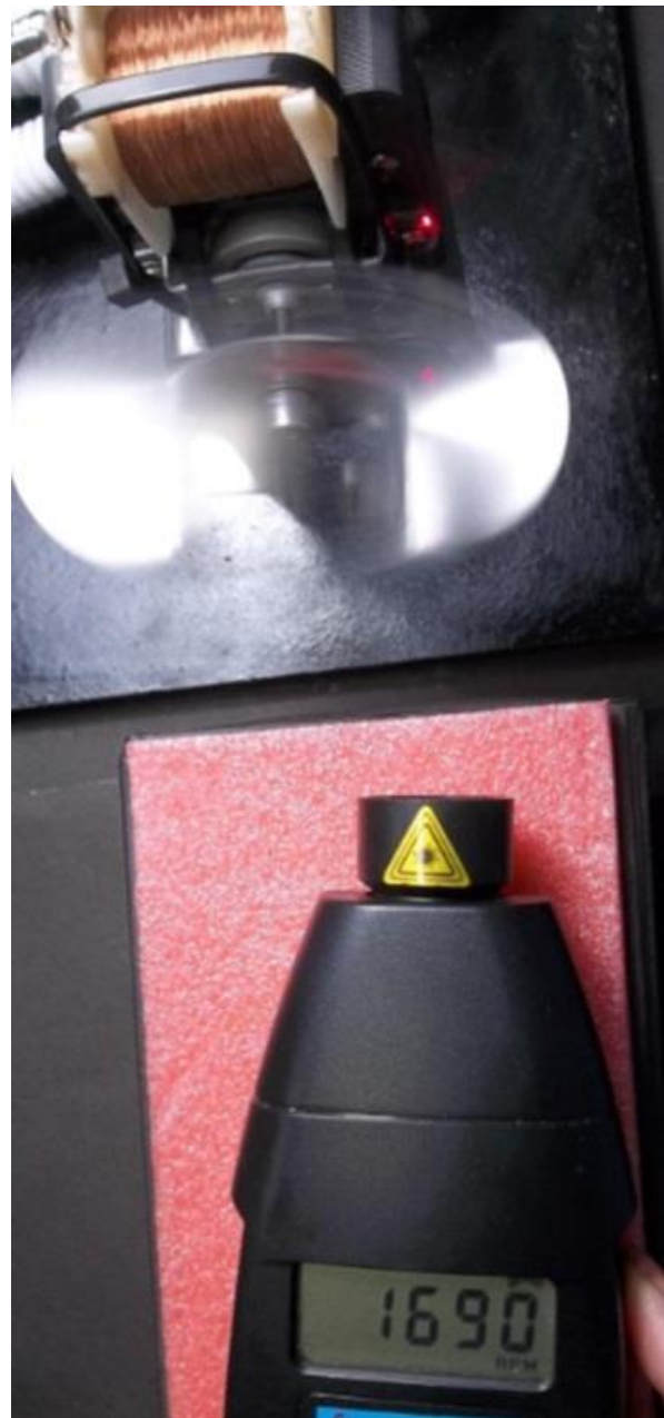
Figure 1: (a) Shaded-pole motor, a type of stopped AC asynchronous single-phase induction motor used in the experiment, with 10.5 (mm) blades used in the experiment; (b) the same motor running at 1690 (RPM) at maximum power of 25 (Watts). Source: self made.
