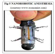
An arbitrary Nano robot consists of up power supply, a camera, legs that allow movement, and various other components based on the function that it is supposed to perform.
