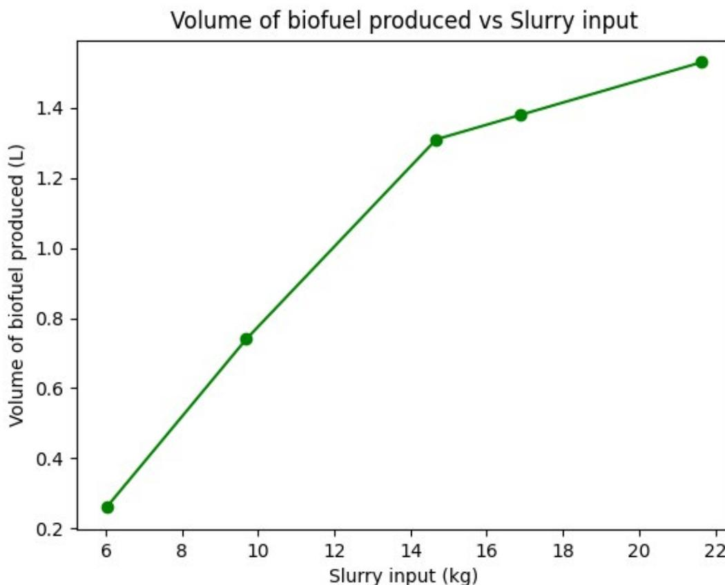
**Figure 4:** Relationship between volume of biofuel produced (L) and the slurry input (kg) for almond fruit
