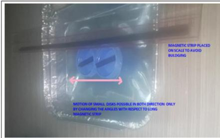
Figure 6: Magnetic strips arrangements in first experiment
