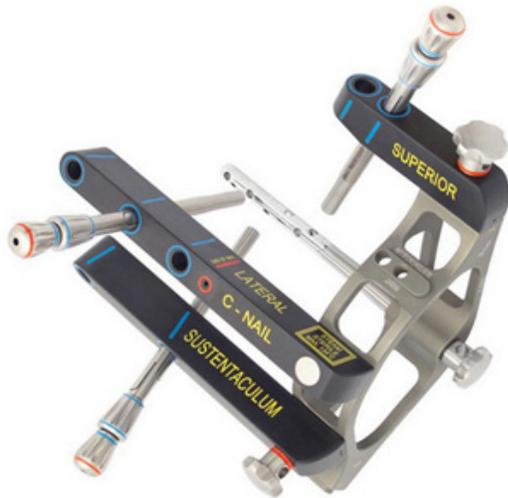
**Figure 1:** C-nail aiming device with three arms (sustentacular, superior, lateral) and the central fixed C-nail having a length of 65 mm, a diameter of 8 mm, and 7 options for locking screws. Two screws are guided by the sustentacular arm into the sustentacular fragment, two by the superior arm into the tuberosity fragment, and 2-3 screws are guided by the lateral arm into the tuberosity fragment and the main anterior process fragment.
