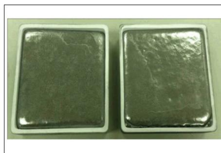
**Figure 8:** Regrown graphite up to 100 mm squares were formed under vacuum in a few hours.
