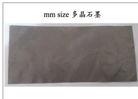
**Figure 5:** The appearance of polycrystalline kish formed by nickel template under vacuum.
