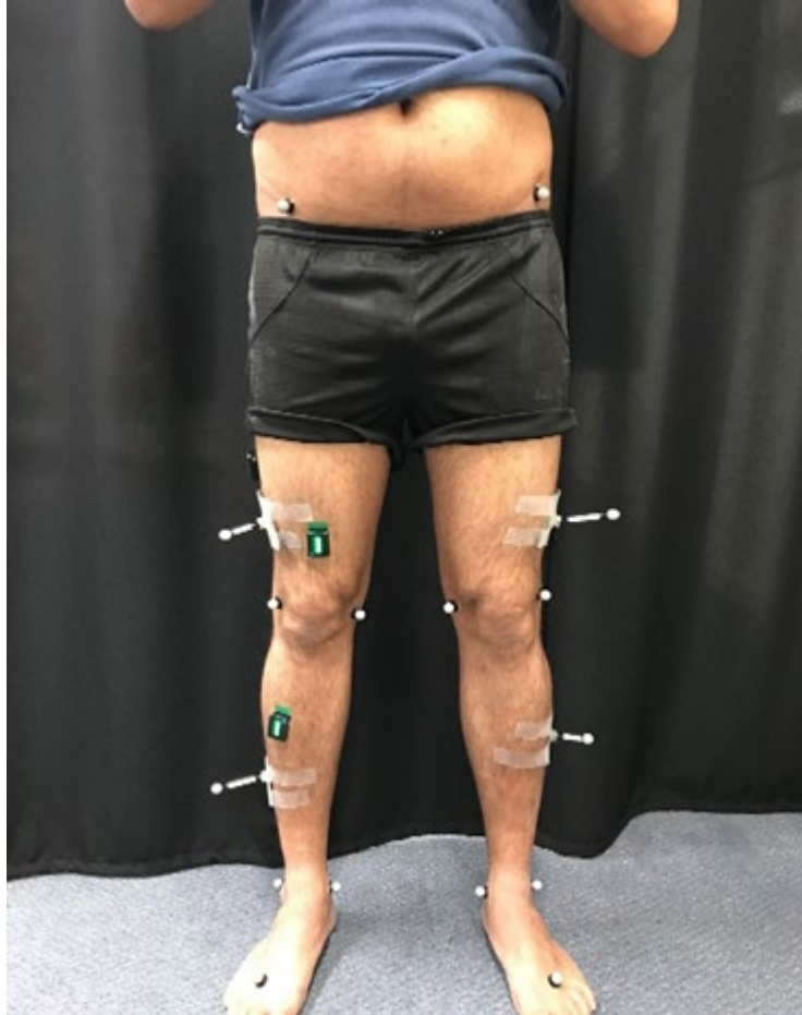
Figure 1: Retro-reflective markers placed according to Vicon Clinical Management System
