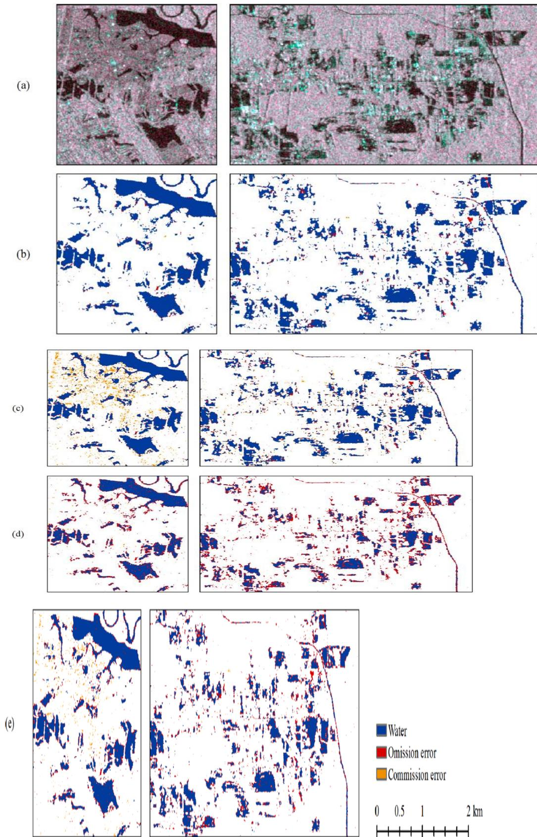
**Fig. 10** (a) The zoomed-in regions' input SAR image. Water extracted with (b) the proposed local thresholding, (c) Otsu's thresholding, (d) Gamma function fitting, and (e) the split-based Kittler-Illingworth technique, with omission and commission errors indicated.
