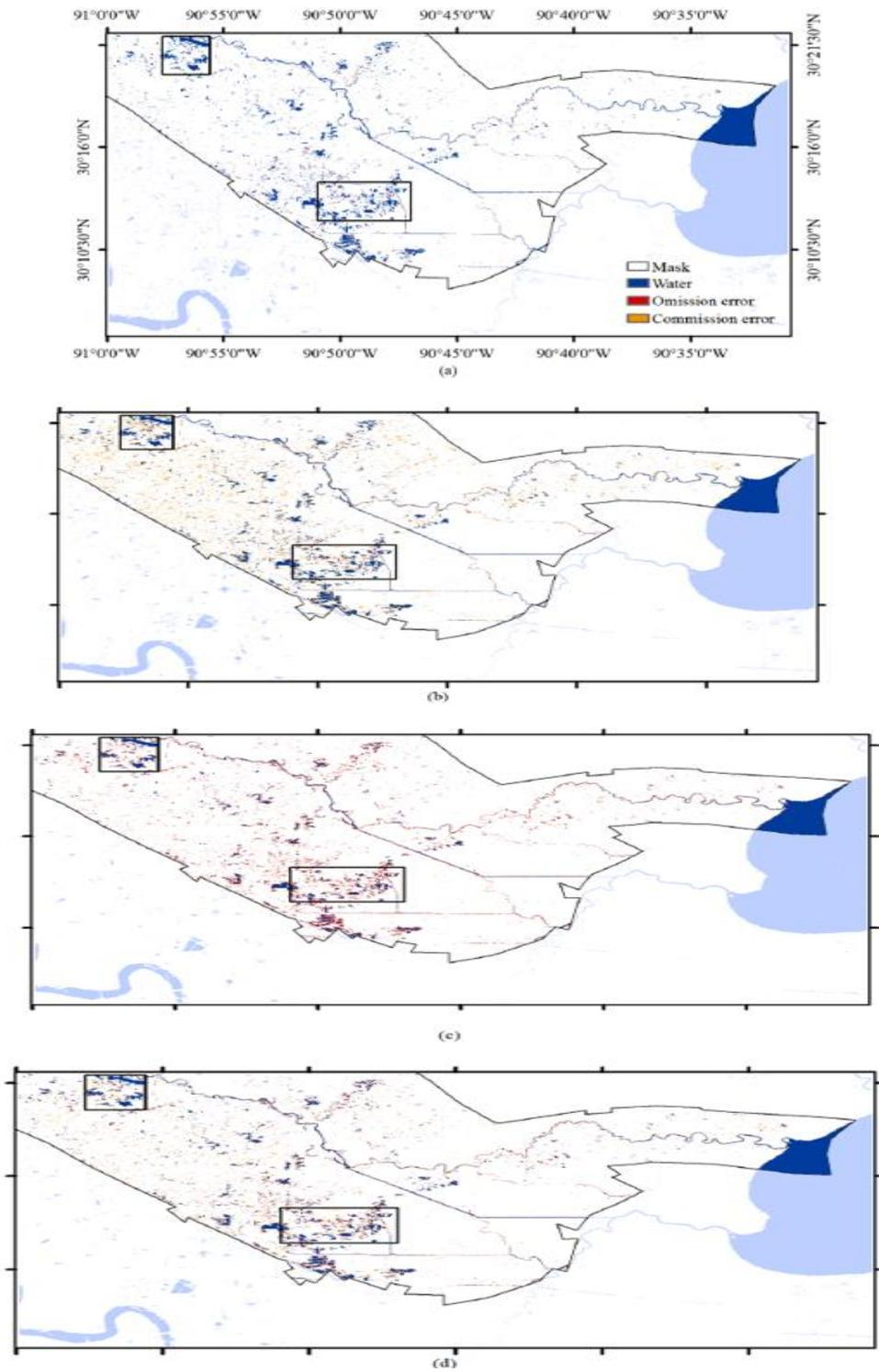
**Fig. 9** Water delineated with (a) the proposed local thresholding, (b) Otsu's thresholding, (c) Gamma function fitting, and (d) the split-based Kittler-Illingworth technique, with omission and commission error underlined and two zoomed-in regions. The mask specifies which aerial images are available [15].
