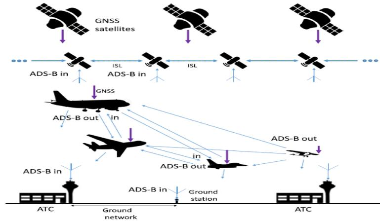
**Fig. 4** LO satellites integration ADS-B hierarchy for ADS-B reception, allowing aircraft communication with Air Traffic Controllers [6].
