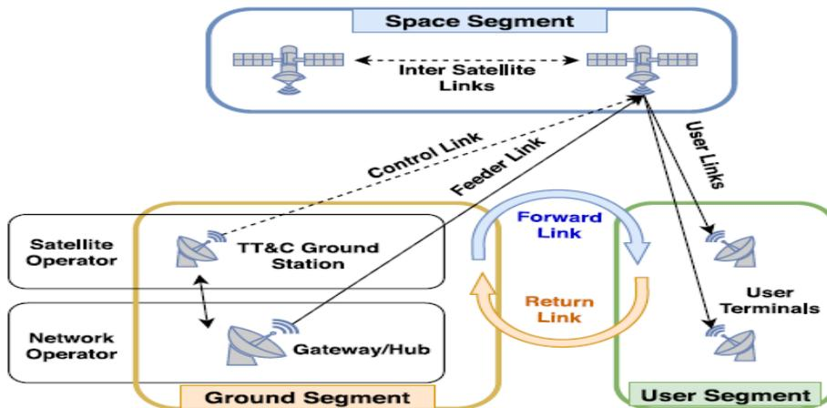
**Fig. 5** SatCom System Architecture [6].
