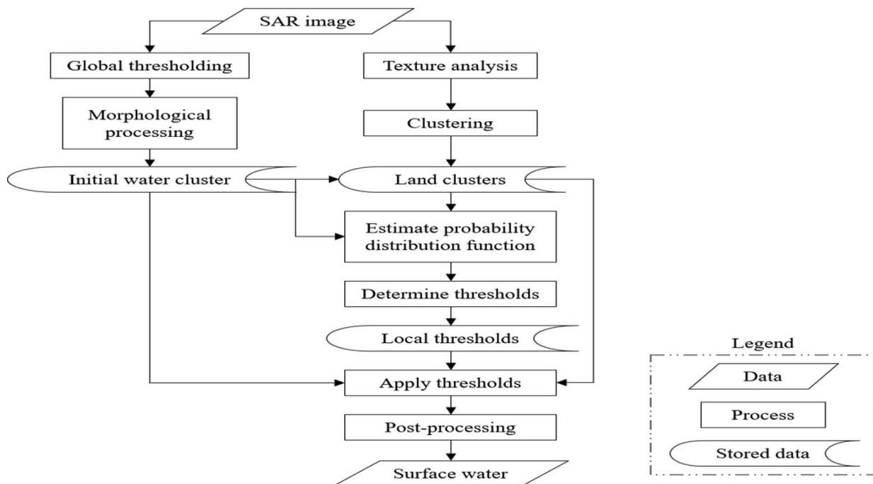
**Fig. 8** The local thresholding method's flow chart [15].
