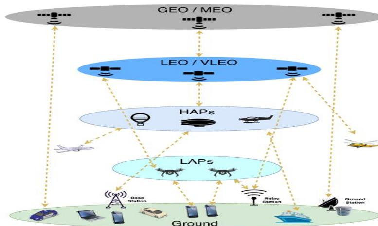
Fig. 3 A multi-layer communications paradigm is depicted schematically. The sub-sections that follow summarize the LAPs, HAPs, and VLEO satellites' advantages and disadvantages [8].
