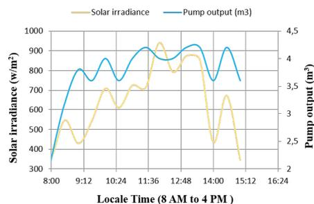
Figure 6: Variation of Solar Irradiance with Pump Output (m3)
