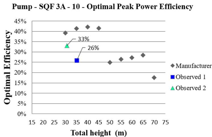
Figure 12: Comparison of the Measured Efficiencies at Different Heights
