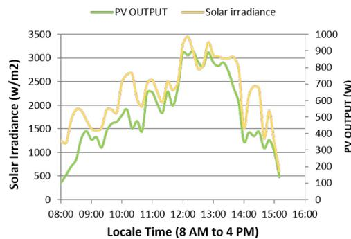
Figure 5: Variation of PV Output with Solar Irradiance
