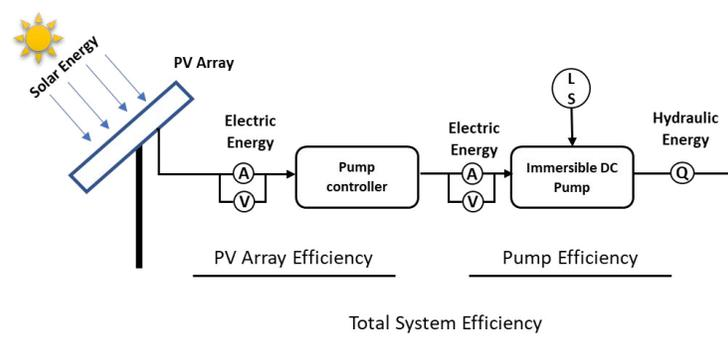
Figure 1: Experiment (Sensors Connection) Scheme
