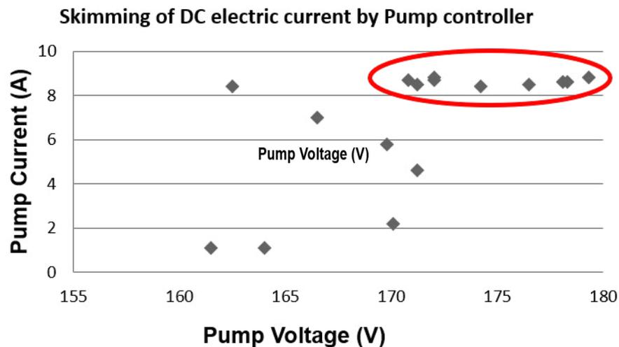
Figure 8: Skimming of DC Electric Current by Pump Controller CU200
