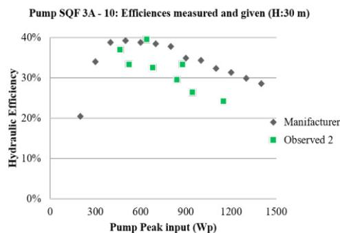
Figure 10: Efficiency with PV Farm of 1.5 kWp
