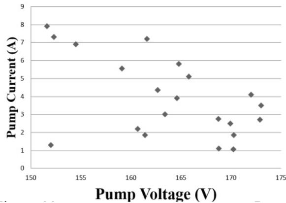
Figure 11: Pump Impedance Voltage (V) VS Current (A) Experiment 2
