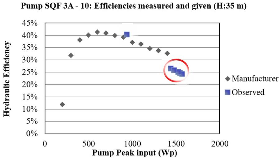
Figure 7: Efficiency Measured for PV 3k WP and given (by the Manufacturer) of the Pump
