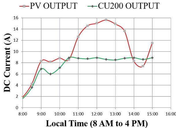
Figure 9: PV Output and Pump Input Variation (12/07/2020)
