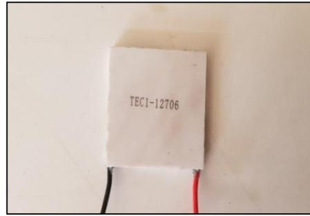
**Figure 2:** Thermo-electric cooler TEC
