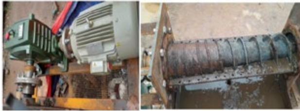
Fig A.1: Motor drive with screw press
