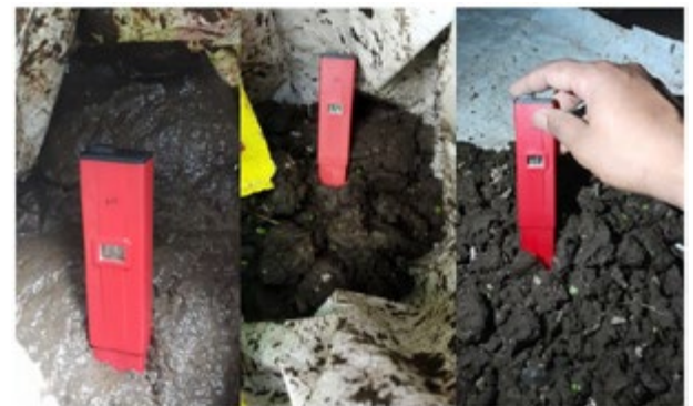
Fig A.5: pH measurement for the sample before and after sundrying
