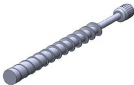
Fig. 7: Motor with screw press (constant pitch & tapered shaft)
