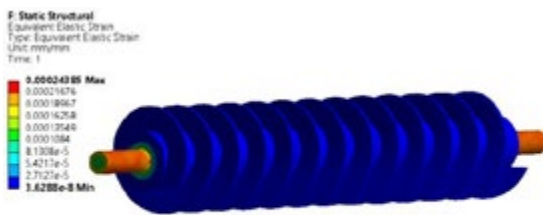
Fig 13: Equivalent Stress - Constant Pitch Screw (Straight shaft)
