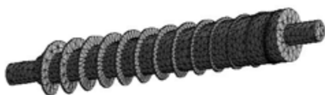
Fig. 9: Meshed Figure - Constant Pitch Screw (Tapered Shaft)
