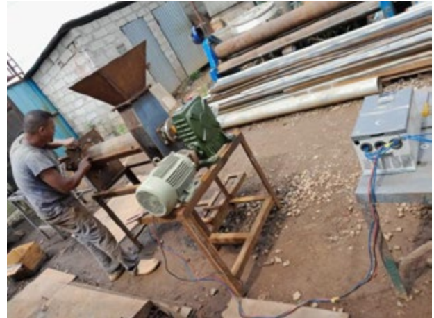
Fig A.4: Assembling work on dewatering machine
