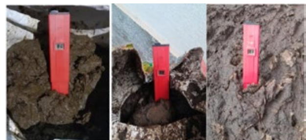
Fig A.6: pH measurement for the pretreatment of sample before dewatering
