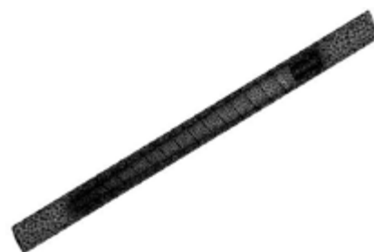
Fig. 11: Fluid Domain - Constant Pitch Screw (Tapered Shaft)
