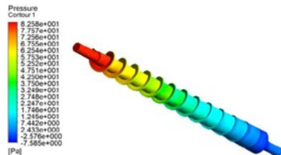
Fig. 27: Pressure Contour - Constant Pitch Screw (Tapered Shaft)
