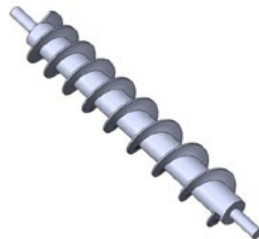
Fig. 4: Variable pitch screw (Straight shaft)
