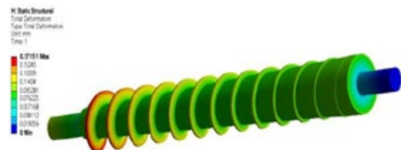
Fig. 24: Total deformation - Constant Pitch Screw (Tapered Shaft)
