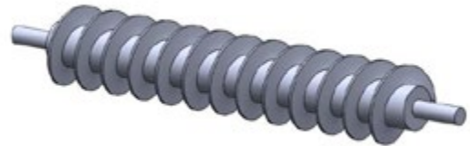
Fig. 3: Constant Pitch Screw (Straight shaft)
