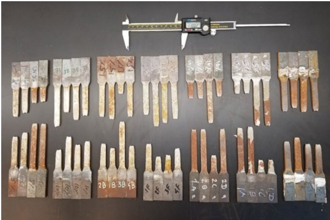
Figure 2: The test samples, subject to various degree of environment-induced damage, subsequent to being deformed and failure in tension.
