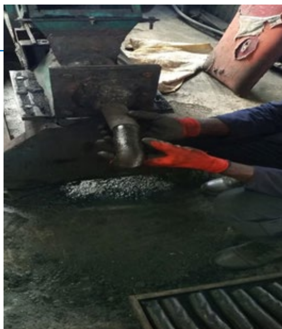
Figure 3: The briquette press machine producing briquettes
