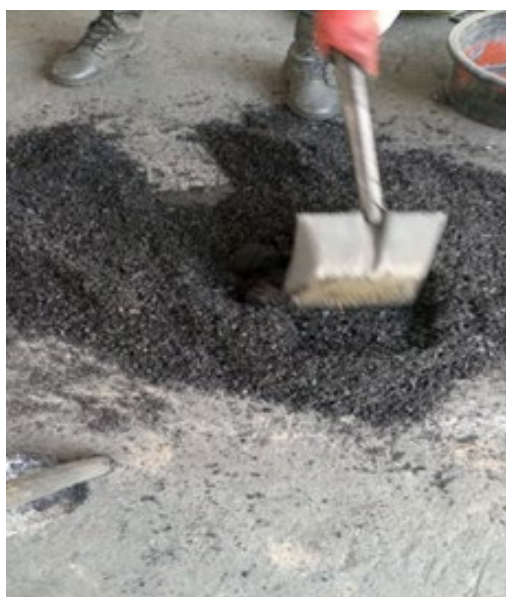
Figure 3: Mixing of the char with binder
