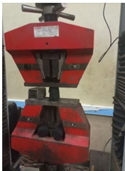
Figure 5: The Compression tester
