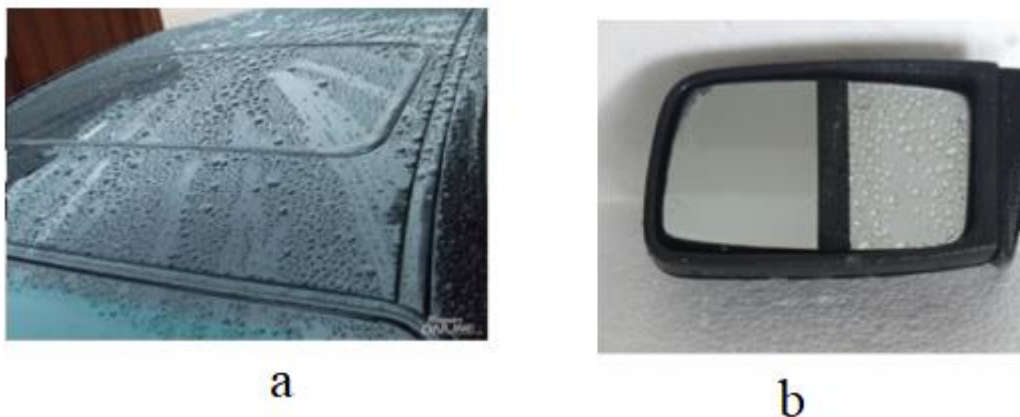
Figure 8: Application of TiO 2 in self-cleaning and anti-fog glass (a) and mirror (b)[7].
