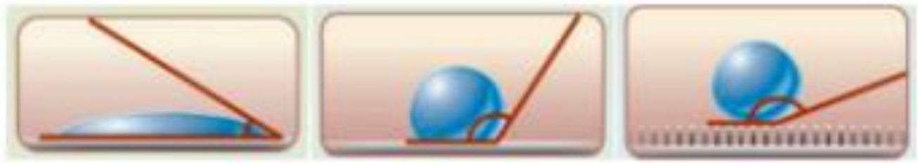
Figure 1: Measurement of stable contact angle in hydrophilic, hydrophobic and superhydrophobic surfaces [2-3].
