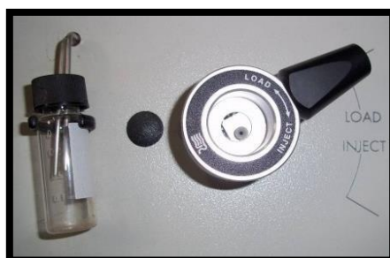
Figure 9: Redone injectors for High Performance Liquid Chromatography
